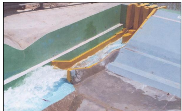
Photo 1 show performance of the ski-jump bucket, Q=2,000 cumec, FRL EL. 1345.0M
